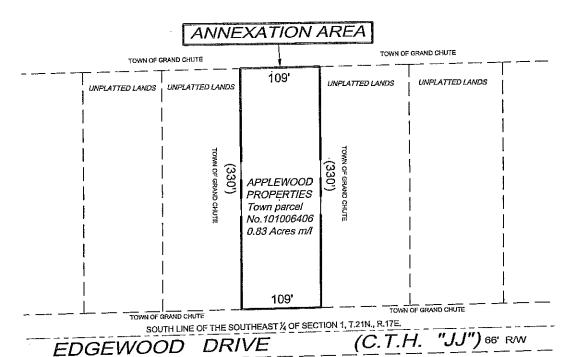
BEARINGS ARE REFERENCED TO THE WISCONSIN COUNTY COORDINATE SYSTEM, OUTAGAMIE COUNTY, SOUTH LINE OF SE 1/4 SECTION 1, T.21N., R.17E.; recorded to bear N89\*14/49\*E
